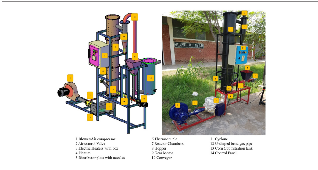
Figure 4. Complete experimental setup of the fluidised bed gasifier with labelled AutoCAD drawing
